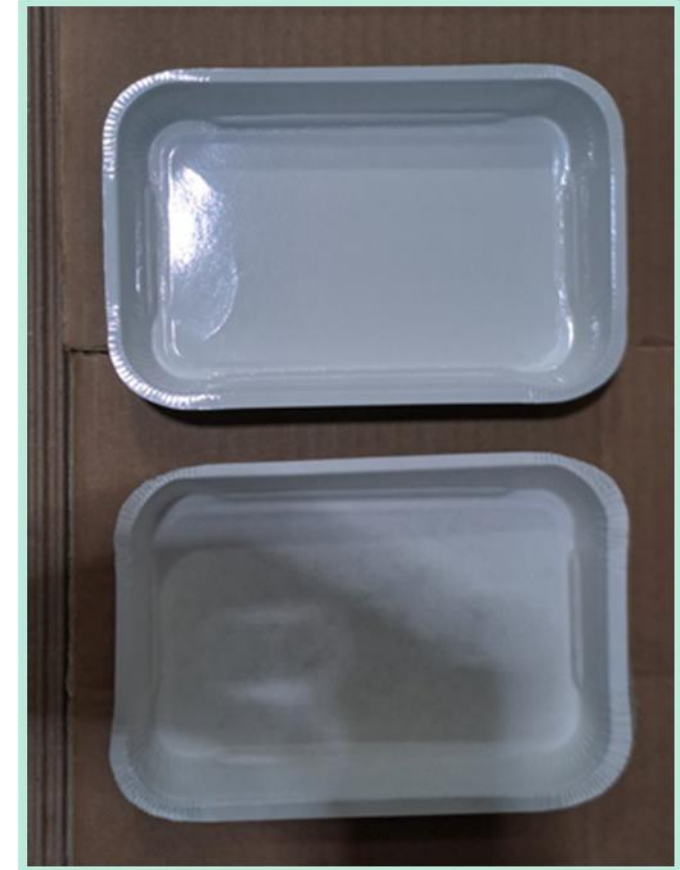
Figure: Paper substrate coated by PBS (left) and thermoformed coated paper
