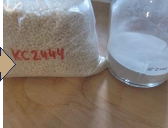
Grinding of thermoplastic granules using cold grinding under nitrogen
