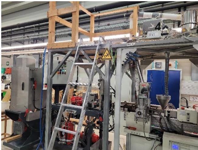
Compounding thermoplastic matrices: Parallel, co-rotating twin screw extruder Brabender DSE20
