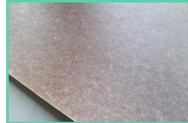
Powder-coated paper substrate using uncondensed lignin
